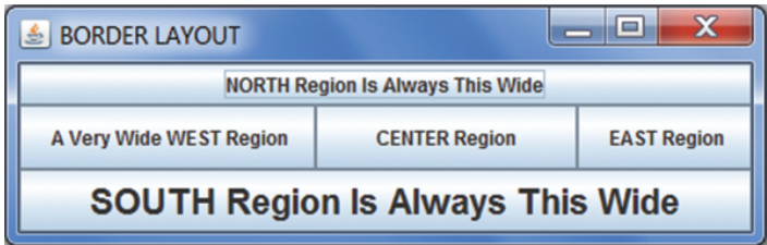
Figure 11.31 The positioning and sizing of the five border layout regions.
